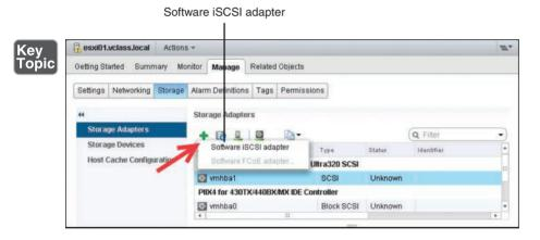
Figure 4-8 Enable a Software iSCSI Initiator
