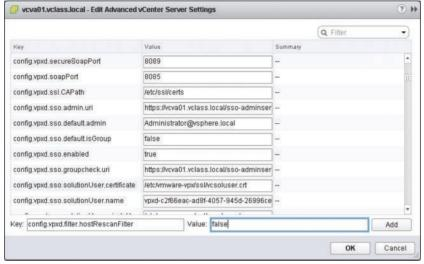
Figure 4-7 Enable a Storage Filter
