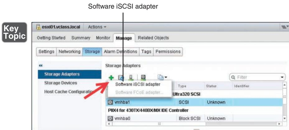
**Figure 4-8** Enable a Software iSCSI Initiator
