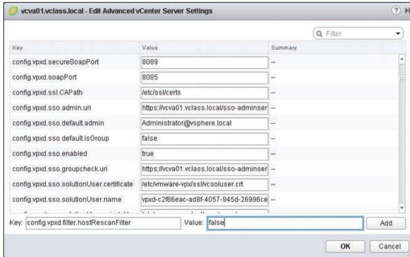
**Figure 4-7** Enable a Storage Filter
